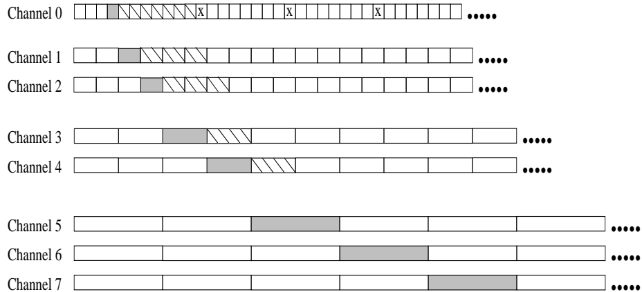
Fig. 2. Segment Size Progression A = \{1, 2, 2, 4, 4, 8, 8, 16, 16, \dots\} . ( K = 8 ; W = 8 )
