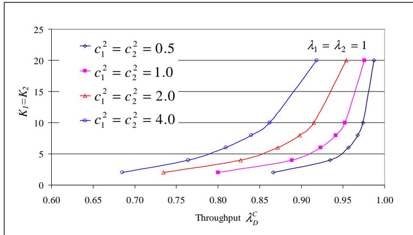
Figure 1.2. Impact of SCVs on  $K_1 + K_2$  required to obtain a given  $\lambda_D^C$
