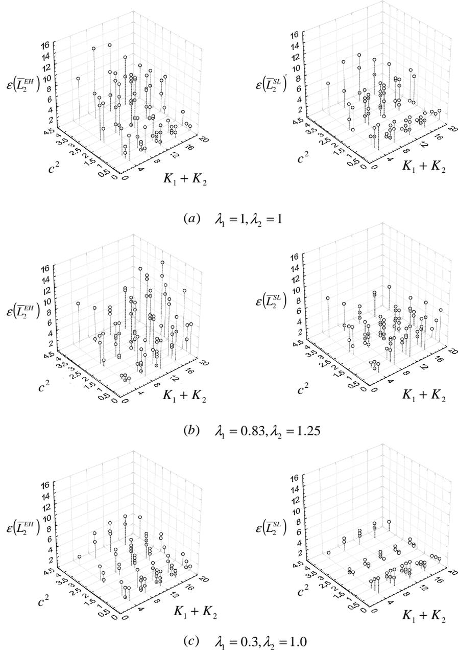
Figure 1.9. Accuracy of approximations for mean queue length ( $\bar{L}_2$ ) at buffer  $B_2$  for different system parameters
