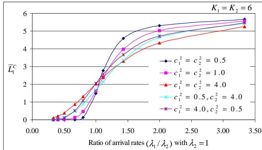
Figure 1.3. Impact of unequal input rates and variabilities on  $\bar{L}_1^C$
