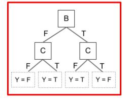
Notice, Y is just a function of B, C: Y = B xor C. Hence, A can be removed and we can build a DT of depth 2 as shown.
