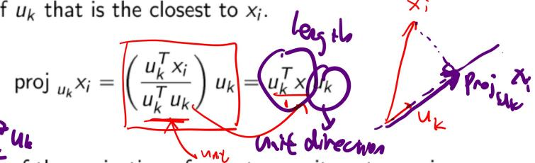
The length of the projection of  $x_i$  onto a unit vector  $u_k$  is  $u_k^T x_i$ .
