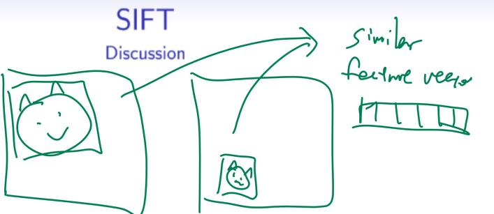
Scale Invariant Feature Transform (SIFT) features are features that are invariant to changes in the location, scale, orientation, and lighting of the pixels.
