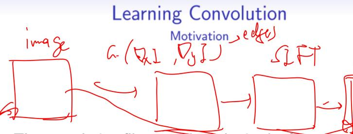
The convolution filters used to obtain the features can be learned in a neural network. Such networks are called convolutional neural networks and they usually contain multiple convolutional layers with fully connected and softmax
