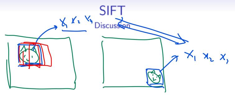
Scale Invariant Feature Transform (SIFT) features are features that are invariant to changes in the location, scale, orientation, and lighting of the pixels.
