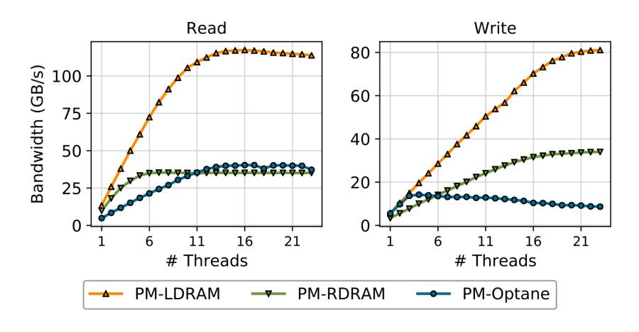
Per-DIMM max read bandwidth: 6.6 GB/s, max write bandwidth: 2.3 GB/s Read/write bandwidth gap is 2.9x for NVM (1.3x for DRAM)
