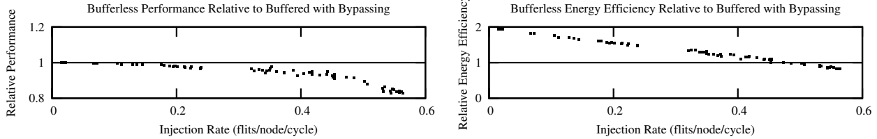
Figure 1. System performance and energy efficiency (performance per watt) of bufferless deflection routing, relative to conventional input-buffered routing (4 VCs, 4 flits/VC) that employs buffer bypassing, in a 4x4 2D mesh. Injection rate (X axis) for each workload is measured in the baseline buffered network.
