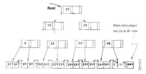
Figure 10.26 After Adding Entry for Leaf Page Containing 38\*
