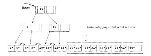
Figure 10.24 Page Split during B+ Tree Bulk-Loading
