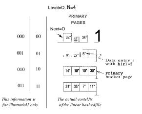
Figure 11.8 Example of a Linear Hashed File
