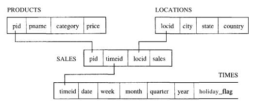
Figure 25.4 An Example of a Star Schema
