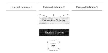
Figure 1.2 Levels of Abstraction in a DBMS
