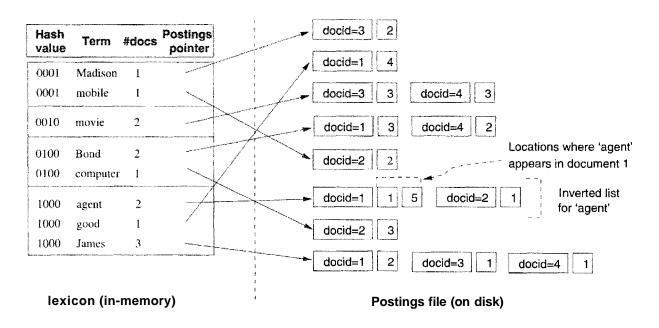
Figure 27.5 Inverted Index for Example Collection
