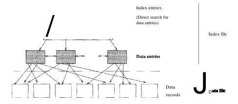
Figure 13.12 Unclustered B+ Tree for Sorting
