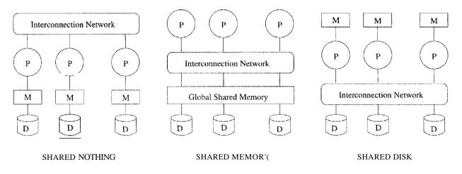
Figure 22.1 PhysicaJ Architectures for Parallel Da.tabase Systems
