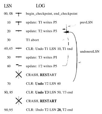
Figure 18.5 Example of Undo with Repeated Crashes
