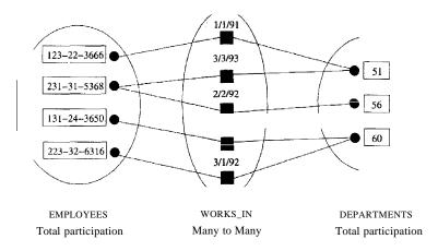
Figure 2.3 An Instance of the Works\_In Relationship Set
