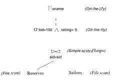
Figure 12.4 Query Evaluation Plan for Sample Query
