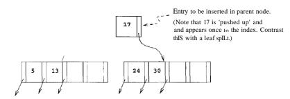
Figure 10.12 Split Index Pages during Insert of Entry 8\*
