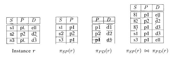
Figure 19.9 Instances Illustrating Lossy Decompositions
