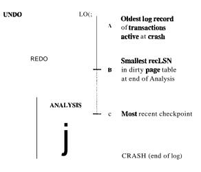
Figure 18.4 Three Phases of Restart in ARIES
