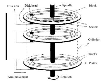
Figure 9.2 Structure of a Disk
