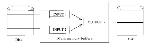
Figure 13.3 Two-'Way Merge Sort with Three Buffer Pages
