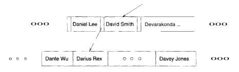
Figure 10.21 Example Illustrating Prefix Key Compression
