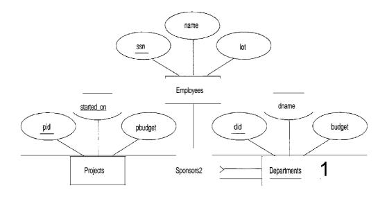
Figure 2.19 Using a Ternary Relationship instead of Aggregation
