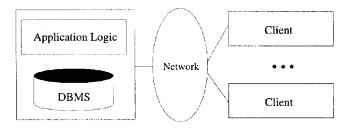
Figure 7.6 A Two-Server Architecture: Thin Clients
