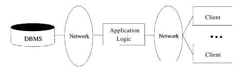
Figure 7.8 A Standard Three-Tier Architecture
